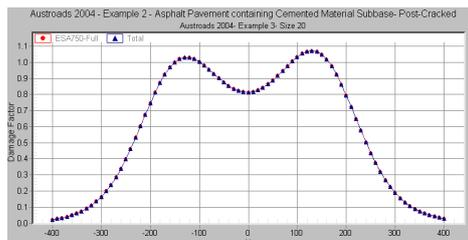
Damage graph shows damage variation across pavement.
